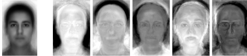
Figure 2. Average face image and the first 5 eigenfaces defining a face space with no image pre-processing.
